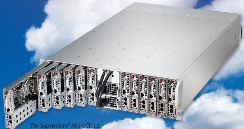
The Supermicro® MicroCloud 12-server node model is shown here.
