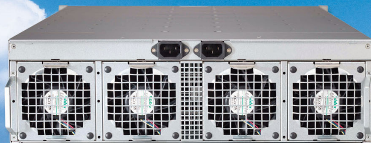
The MicroCloud system utilizes Redundant 1620W Platinum Level (94%) high-efficiency power supplies and sophisticated cooling zone controls for a Green energy profile.
